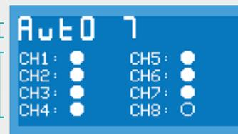
**Active channels:** the load cell is connected
